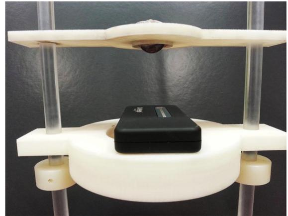
Fig. 3: Experimental setup for determining the RFID read range through Porcine Eyes
