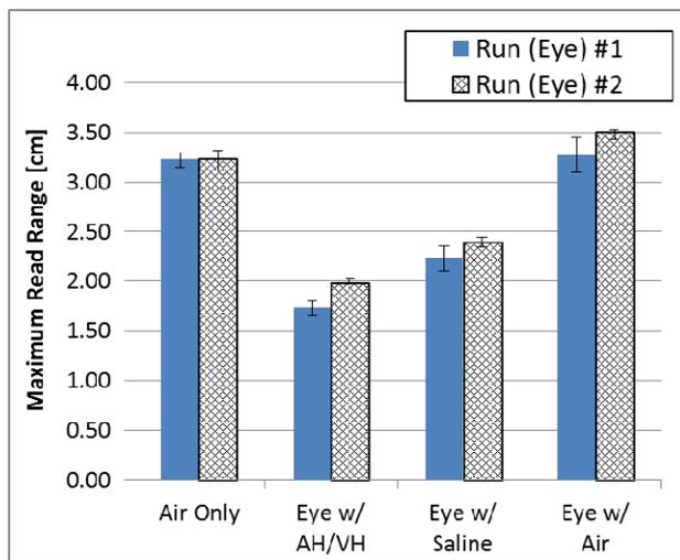
Fig. 4: Tested read ranges for the LF (125 kHz) system
