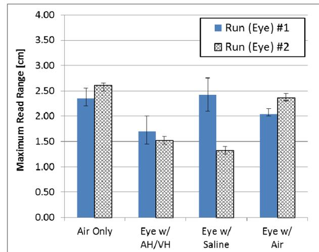
Fig. 6: Tested read ranges for the UHF (~900 MHz) system
