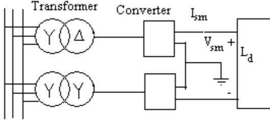
Fig.2. Main components of SMES System
