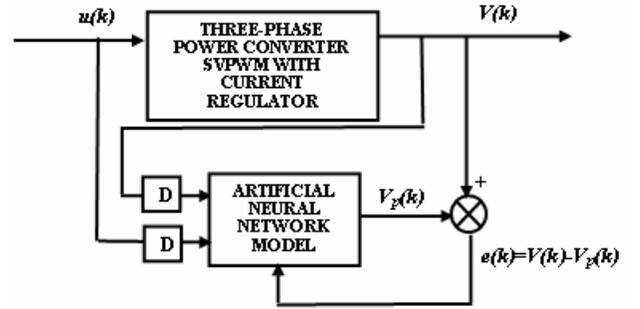
Figure 5. The diagram for Training of the Plant Model
