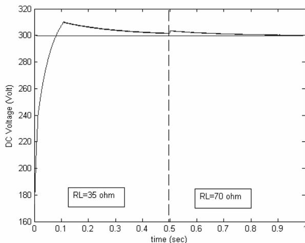
Figure 12. Time Response of DC Voltage respect to the load change
