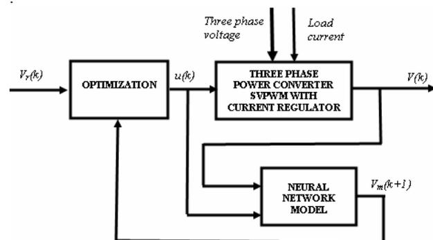
Figure 2. Neural Predictive Control of Three-Phase Converter SVPWM with Current Regulator
