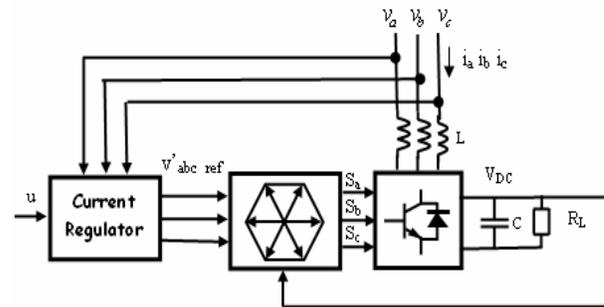
Figure 1. Three-Phase Power Converter SVPWM with Current Regulator
