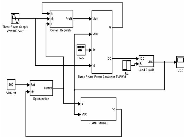
Figure 11. Simulink Diagram of Neural Predictive Control
