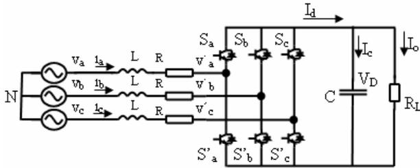
Figure 7. Three-phase Power Converter Circuit
