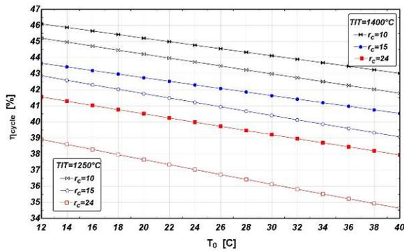
Figure 5. Effect of compressor inlet air temperature on RGT efficiency in different  $r_c$  and TIT ( $\phi_0=60\%$ )
