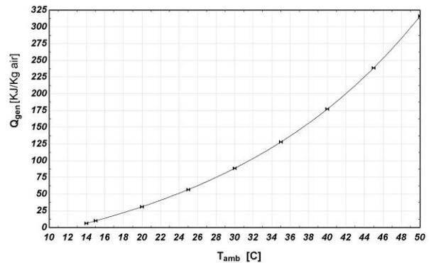
Figure 7. ARC required energy as a function of ambient temperature for providing specified inlet cooling ( $T_0=12^\circ\text{C}$ ,  $\phi_{amb}=60\%$ ,  $\phi_0=60\%$ )
