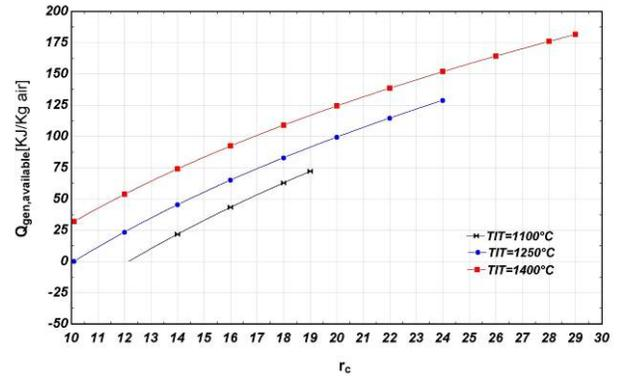
Figure 18. Thermal energy of RGT exhaust gases as a function of  $r_c$  and TIT ( $T_0=12^{\circ}C$ ,  $\phi_0=60\%$ )
