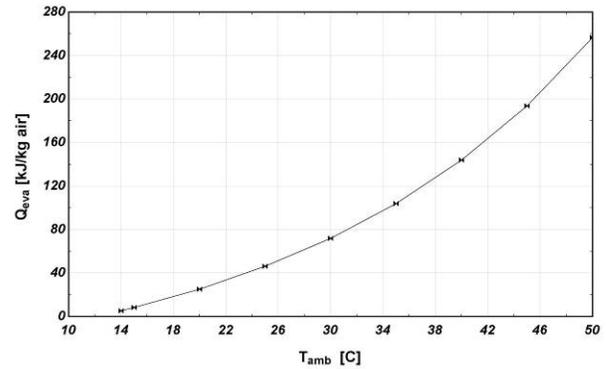
Figure 6. Required cooling capacity for inlet air cooling as a function of ambient temperature ( $T_0=12^\circ\text{C}$ ,  $\phi_{amb}=60\%$ ,  $\phi_0=60\%$ )
