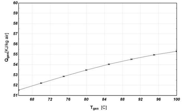
Figure 12. ARC required energy as a function of  $T_{gen}$  for providing specified inlet cooling ( $T_{amb}=25^{\circ}\text{C}$ ,  $T_0=12^{\circ}\text{C}$ ,  $\phi_{amb}=60\%$ ,  $\phi_0=60\%$ )
