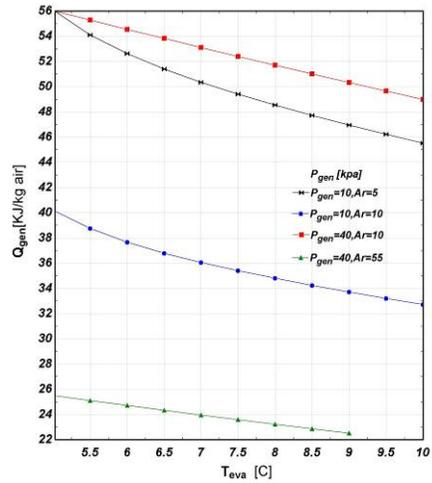
Figure 15. EARC required energy as a function of  $T_{eva}$ ,  $P_{gen}$  and  $A_r$  for providing specified inlet cooling ( $T_{amb}=25^{\circ}C$ ,  $T_0=12^{\circ}C$ ,  $\phi_{amb}=60\%$ ,  $\phi_0=60\%$ )
