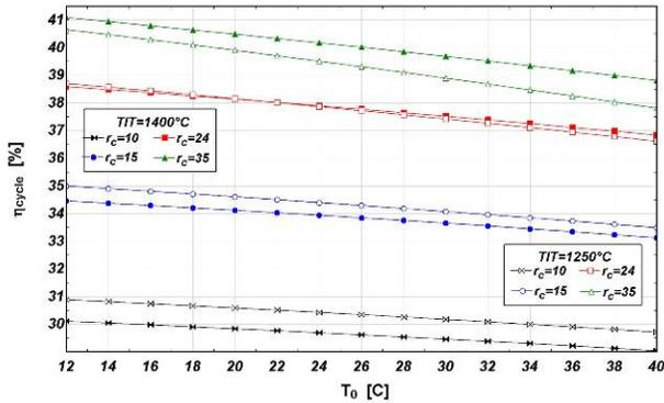
Figure 4. Effect of compressor inlet air temperature on SGT efficiency in different  $r_c$  and TIT ( $\phi_0=60\%$ )
