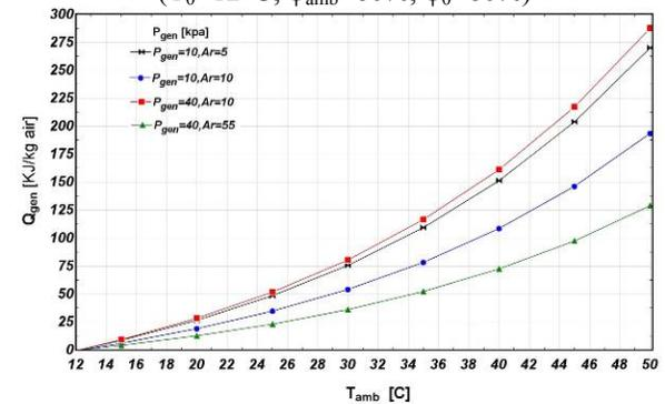
Figure 8. EARC required energy as a function of ambient temperature,  $P_{gen}$  and  $A_r$  for providing specified inlet cooling ( $T_0=12^\circ\text{C}$ ,  $\phi_{amb}=60\%$ ,  $\phi_0=60\%$ )
