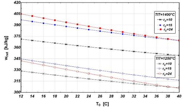
Figure 3. Effect of compressor inlet air temperature on RGT specific work in different  $r_c$  and TIT ( $\phi_0=60\%$ )
