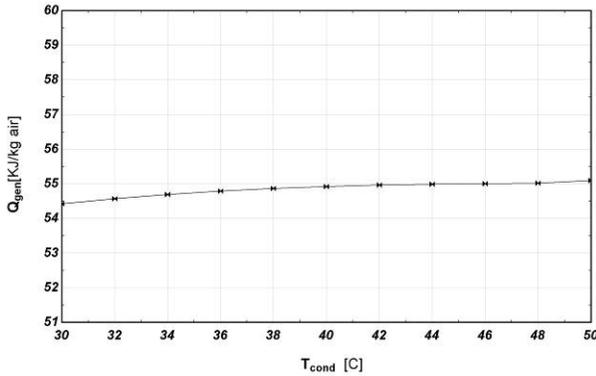
Figure 10. ARC required energy as a function of  $T_{cond}$  for providing specified inlet cooling ( $T_{amb}=25^{\circ}\text{C}$ ,  $T_0=12^{\circ}\text{C}$ ,  $\phi_{amb}=60\%$ ,  $\phi_0=60\%$ )
