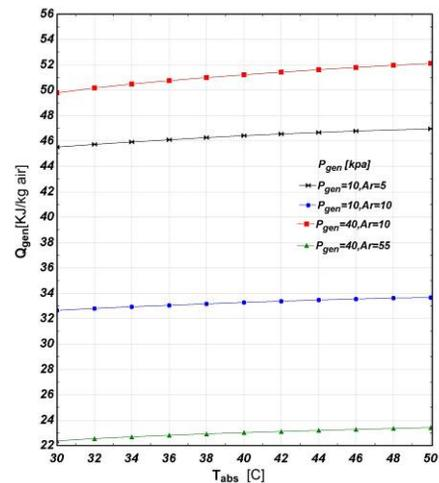
Figure 13. EARC required energy as a function of  $T_{abs}$ ,  $P_{gen}$  and  $A_r$  for providing specified inlet cooling ( $T_{amb}=25^{\circ}\text{C}$ ,  $T_0=12^{\circ}\text{C}$ ,  $\phi_{amb}=60\%$ ,  $\phi_0=60\%$ )
