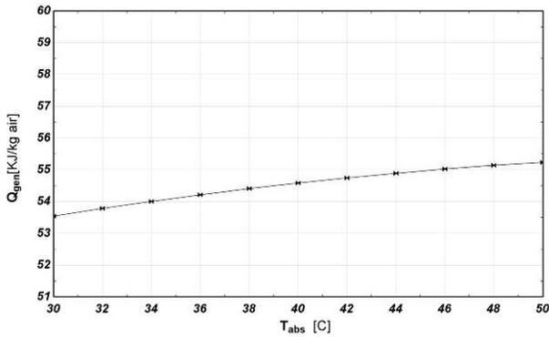
Figure 9. ARC required energy as a function of  $T_{amb}$  for providing specified inlet cooling ( $T_{amb}=25^{\circ}\text{C}$ ,  $T_0=12^{\circ}\text{C}$ ,  $\phi_{amb}=60\%$ ,  $\phi_0=60\%$ )
