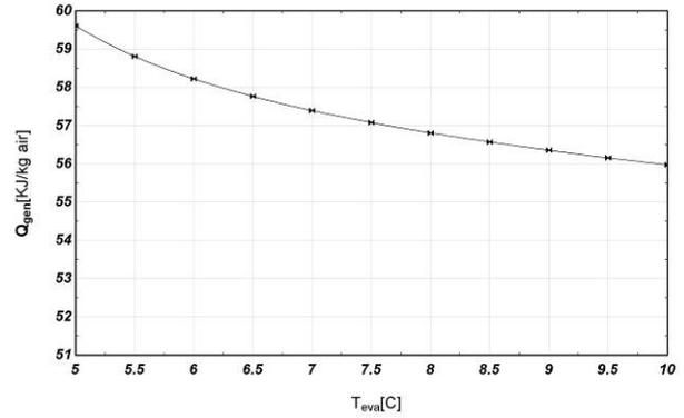
Figure 11. ARC required energy as a function of  $T_{eva}$  for providing specified inlet cooling ( $T_{amb}=25^{\circ}\text{C}$ ,  $T_0=12^{\circ}\text{C}$ ,  $\phi_{amb}=60\%$ ,  $\phi_0=60\%$ )
