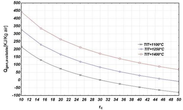
Figure 17. Thermal energy of SGT exhaust gases as a function of  $r_c$  and TIT ( $T_0=12^{\circ}C$ ,  $\phi_0=60\%$ )
