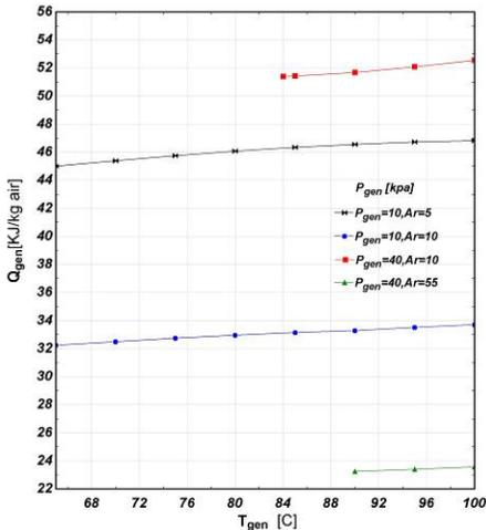
Figure 16. EARC required energy as a function of  $T_{gen}$ ,  $P_{gen}$  and  $A_r$  for providing specified inlet cooling ( $T_{amb}=25^{\circ}C$ ,  $T_0=12^{\circ}C$ ,  $\phi_{amb}=60\%$ ,  $\phi_0=60\%$ )
