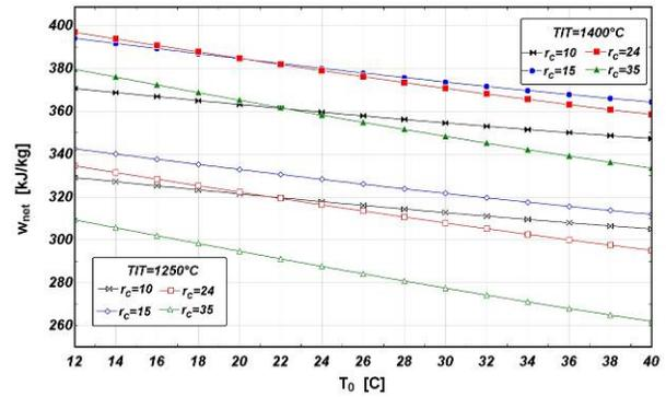
Figure 2. Effect of compressor inlet air temperature on SGT specific work in different  $r_c$  and TIT ( $\phi_0=60\%$ )
