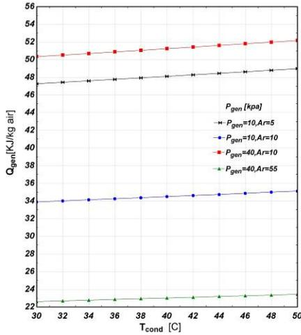
Figure 14. EARC required energy as a function of  $T_{cond}$ ,  $P_{gen}$  and  $A_r$  for providing specified inlet cooling ( $T_{amb}=25^{\circ}C$ ,  $T_0=12^{\circ}C$ ,  $\phi_{amb}=60\%$ ,  $\phi_0=60\%$ )
