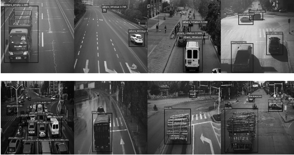
Figure 5. Vehicle detection effect in multiple environments during the day.
