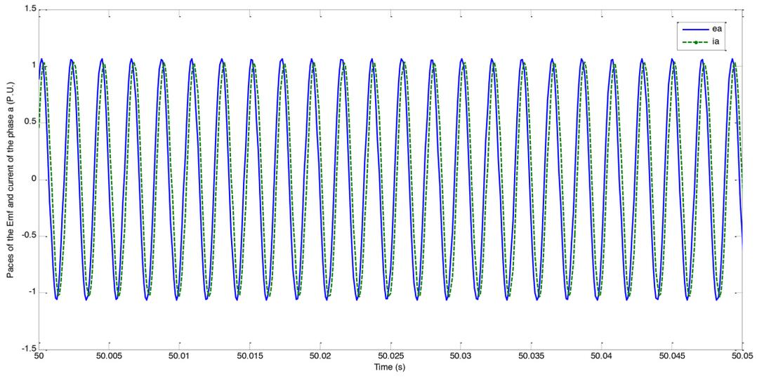
Figure 12. Paces of the generator phase's induced electromotive force and current of the phase 'a' in versus time.
