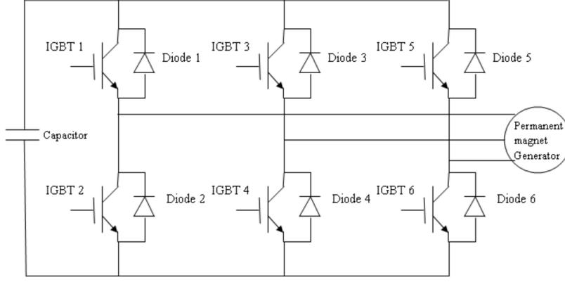
Figure 4. AC–DC converter structure.
