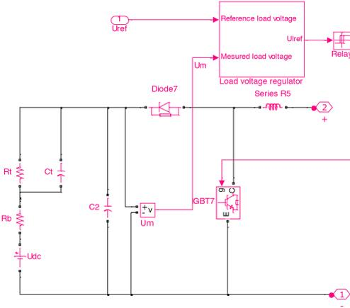
Figure 7. DC-DC inverter regulating battery load voltage by pulse width modulation.
