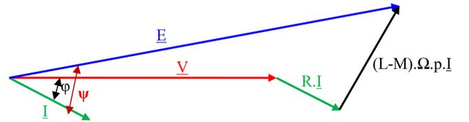
Figure 2. Vector diagram of synchronous generator.
