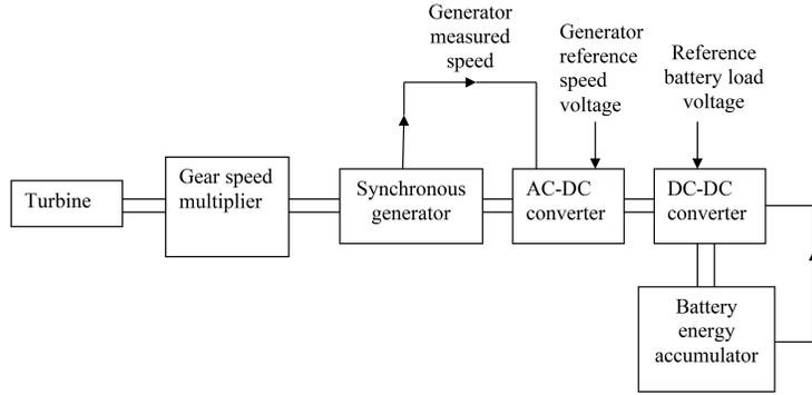
Figure 1. Wind energy generation chain structure.
