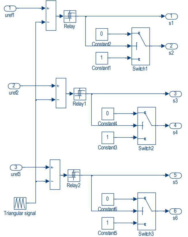
Figure 5. Model of the control signal generator.
