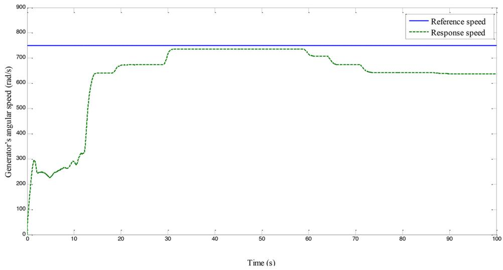
Figure 10. Evolution of the rotational angular speed of the generator.
