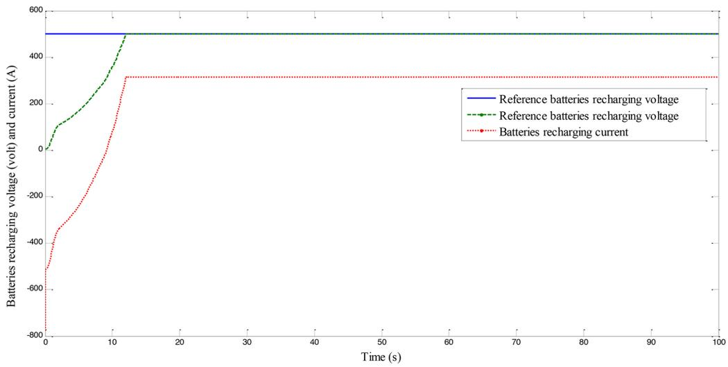
Figure 13. Evolution of battery charging voltage and current.
