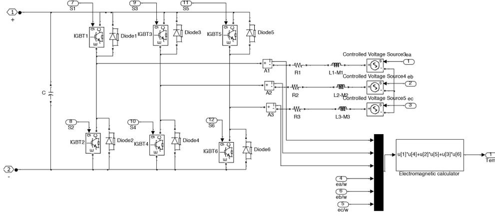
Figure 6. Model of the generator-converter.
